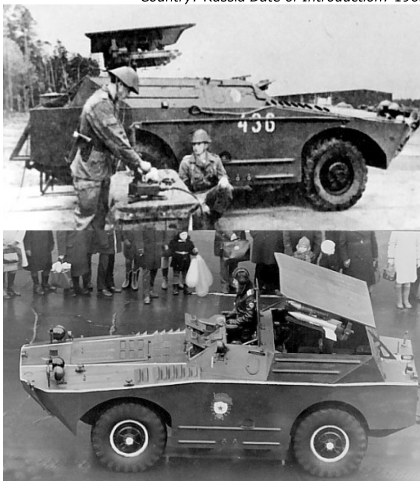
Top: DDR (East German Army) 9P110 with portable launch controller set up on a table. This controller could be offset from the launcher itself for concealment and/or protection of the operator. Above: Soviet/Russian 9P110 missile carrier during one of the yearly parades in Moscow. The launcher rails and cover had a limited left and right powered rotation to give some flexibility to placement of the vehicle. (Photos: Author's collection)
