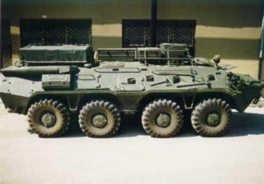
The BTR-80 MPAEJ (Technical Barrier Armored Response Vehicle) has a primary function of the reconnaissance of artificial barriers, devastated ground and the removal of such barriers. It is also designed to have a secondary mission of the protected movement of specialist personnel and their equipment.
