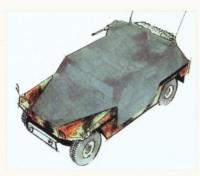
Grey marked area protected against: 7.62 mm BALL from 30 m 5.56 mm BALL from 30 m 7.62 mm steelcore from 100 m
