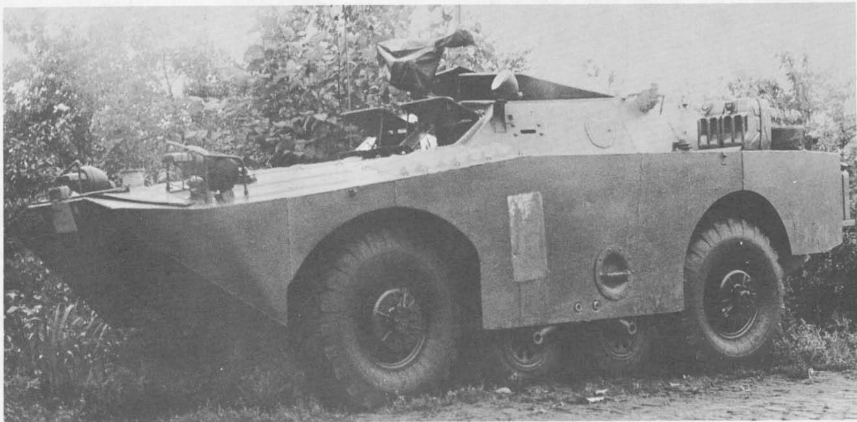
BRDM with rough terrain wheels in lowered position.
