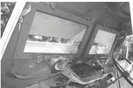
*RUC FV1609, note wipers fitted to windcreens not to body.*
