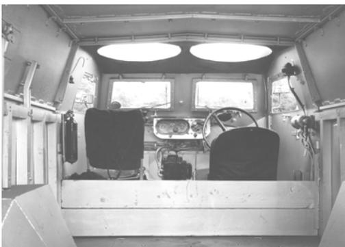
*Note: Strut on left for securing the roof, bent fuel vent pipe on left being used to hold a bunch of keys, clamp on right door is to lock flap when closed as the proper catch at the top is broken, driver's door handle wedged in pipes on right that supply tyre pump, air filter and clutch reservoir.*
