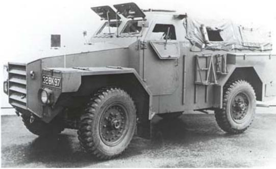
*Later version of FV1609 with a single slope on the front cab armour*
