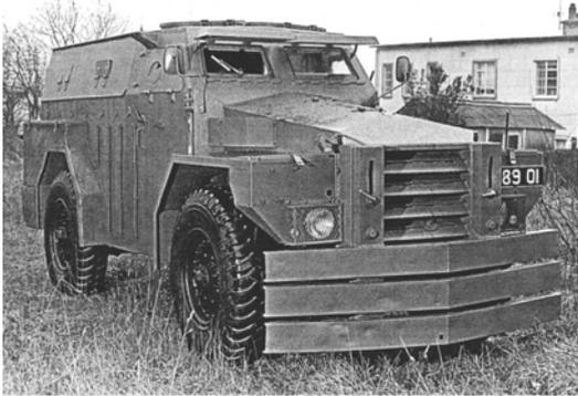
*2989 01 with FV1611 type headlight covers and number plate now displayed on near side.*
