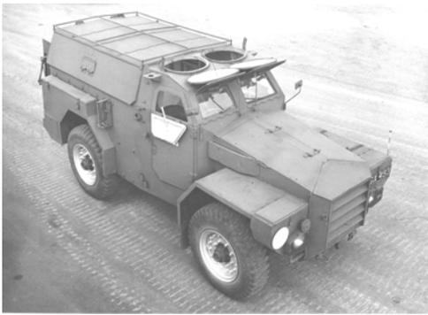
*Humber RGX 493 now with the FV337270 bolt-on roof.*
