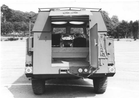
*RGX 493 from the rear. Note the winch that indicates this vehicle predates the 20 prototype vehicles, which were all FV1609(A) i.e. without winch.*
