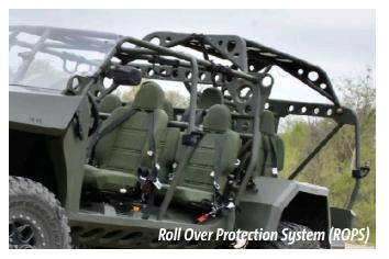
A highly efficient **Roll Over Protection System (ROPS)** features 4130 chromoly tubing to deliver low-mass, high-strength **protection for up to nine occupants.**
