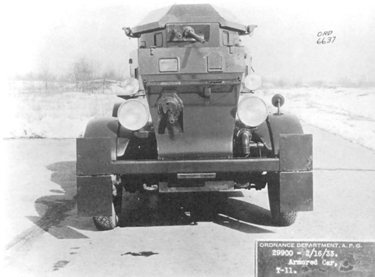
Remarks: Completed in 1932, the pilot T11 was tested at Aberdeen Proving Ground from January to July of 1933. As delivered by FWD, the car had several problems including mechanical failures due to insufficient strength of the rear end. Despite the problems, an order for six cars was issued which the Marmon-Herrington Company would complete.
