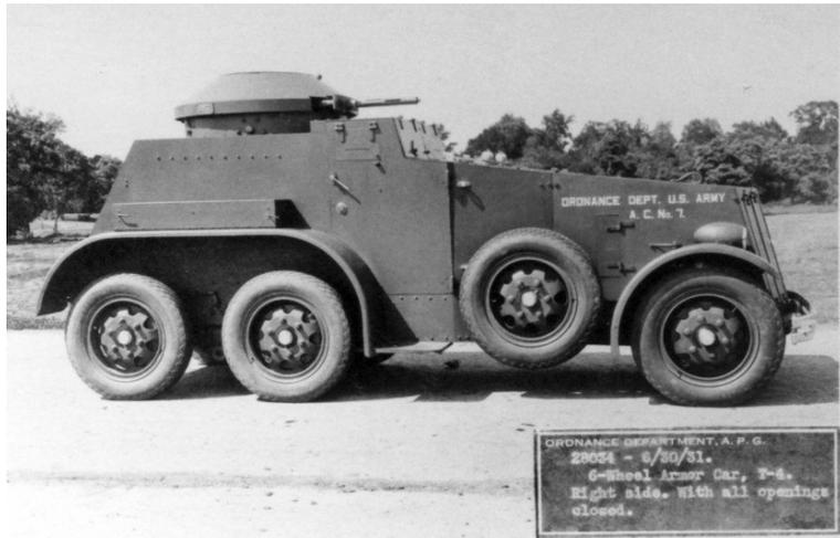
Remarks: Designed and built by James Cunningham Sons and Company, two T4 Armored Cars were completed and tested until 1934 when the design was type classified as the M1 Armored Car. After classification, an additional ten cars were completed. While the cars' performance on hard surfaces was adequate, the non-driving front axle and length of the vehicle (even with the spare wheels able to rotate on stub axles) made cross-country travel marginal at best.
