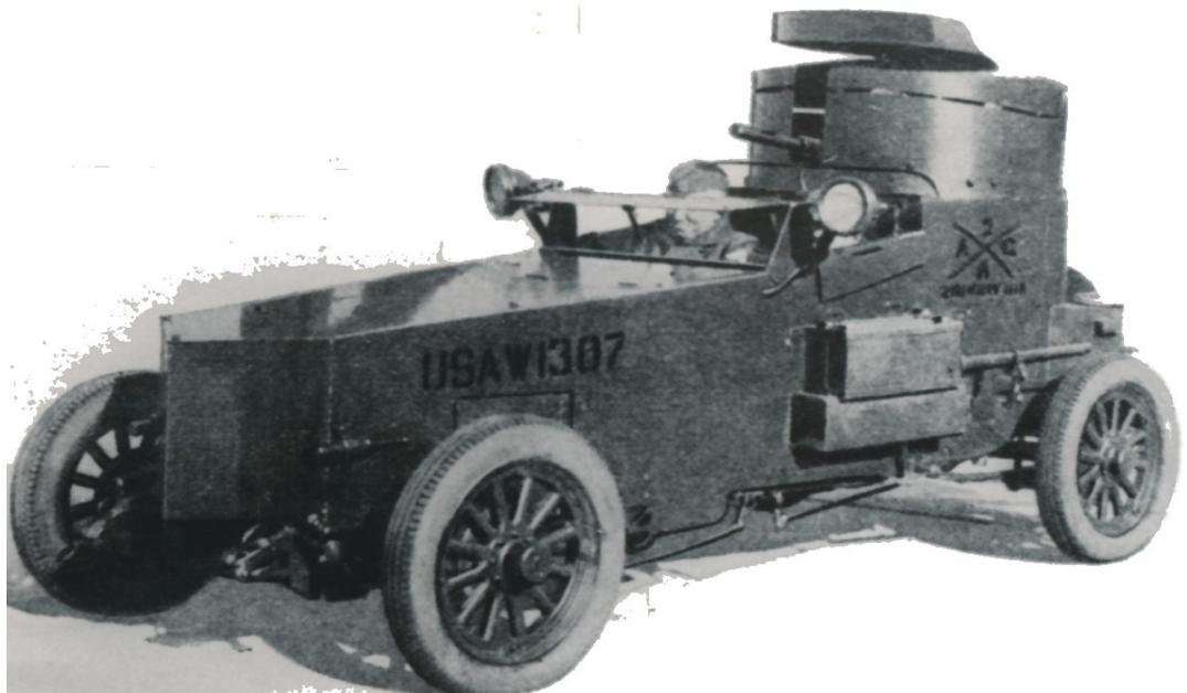
Below: One of the T10 Armored Cars as it appeared in the early 1930s at the US Army Cavalry School. Although there is a large square exterior fuel tank added to the left side of the vehicle, it has the same thick spoked wheels.
