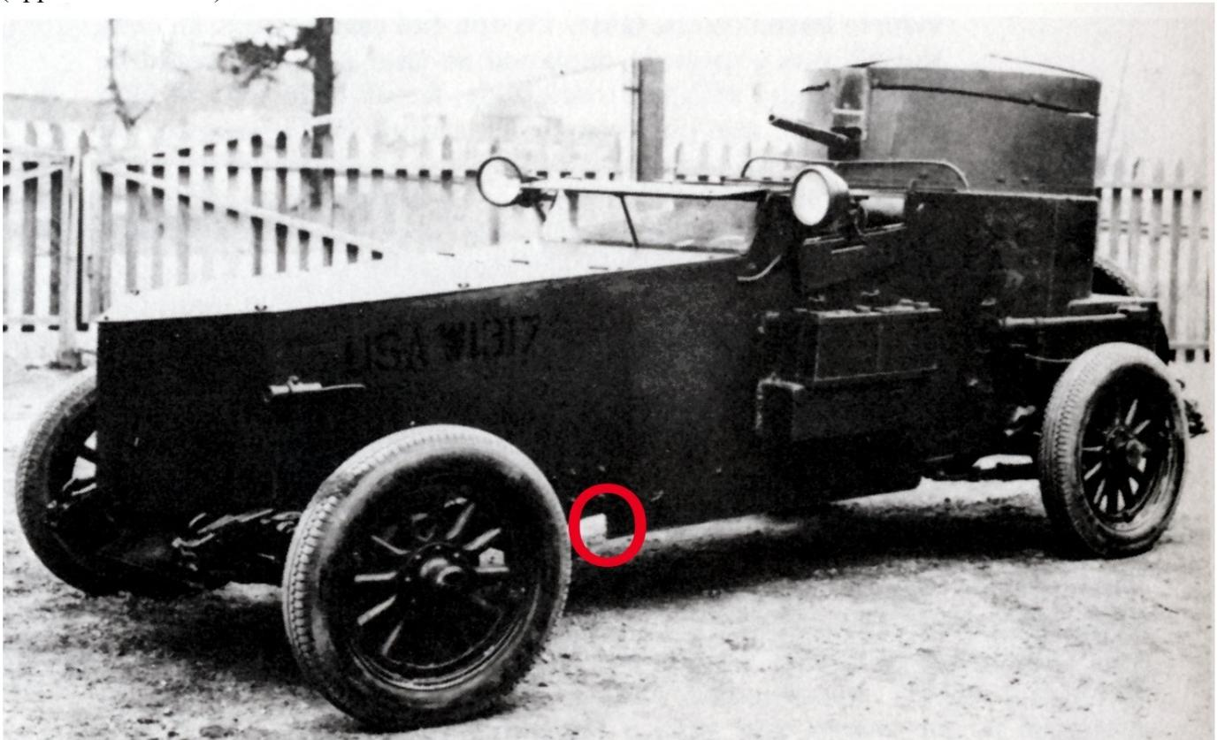
**1932 Armored Car T6 (2<sup>nd</sup> Version).** Although still on the Quartermaster Corp's 1 1/4-ton 4x4 chassis, the second T6 used the armor from the T7 series of Armored Cars and while it carried the same T6 designation had a new set of War Department numbers with one vehicle being W-6011. Photographic evidence suggests that at least two and possibly three vehicles were converted to the revised T6. I don't know what the War Department numbers might be.
