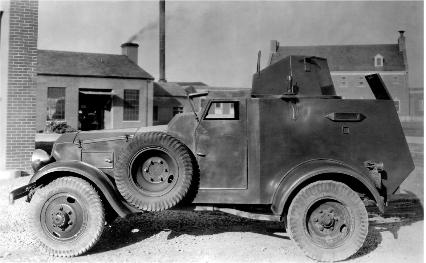
Below: What appears to be an early modification of a T7 body to a T6 style chassis. This might be the early T6-4WD being refurbished in 1930, a second similar modification seems to be in the background.
