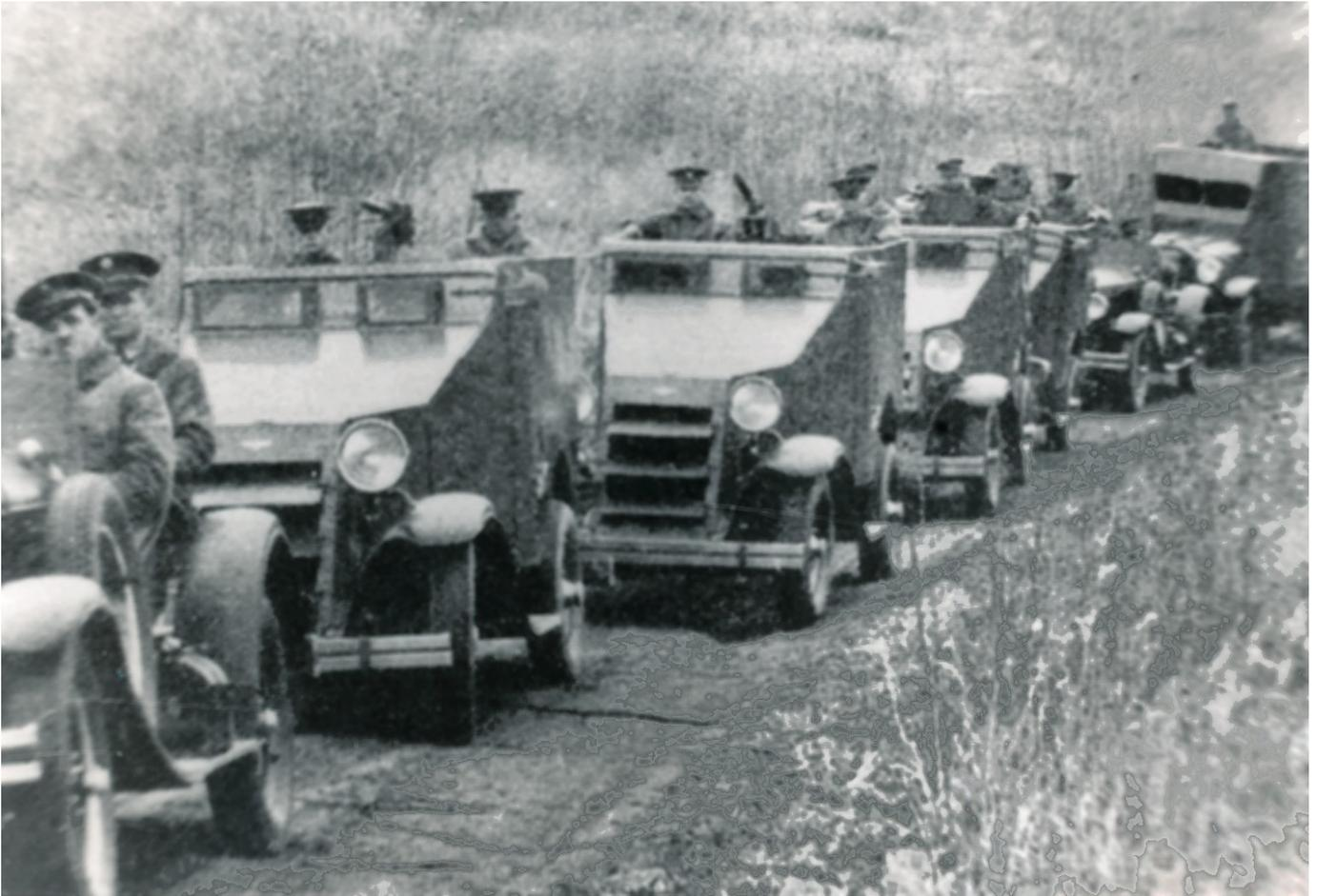
Above: The four Armored Car T2s along with what appear to be both of the Armored Car Light T1s. The last vehicle in line is a Quartermaster truck fitted with armor plate to act as an Armored Personnel Carrier. The number of this vehicle if any, is unknown.
