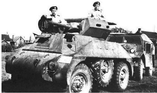
Above: The single completed Hamilton Bridge Wheeled Tank. The two spares were mounted on free wheeling hubs to help keep the vehicle from being "high-centered". (Author's Collection).
