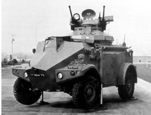
**Remarks:** A co-development of Dassault and Panhard, the M-3 VDA carries the TA-20 turret fitted with twin Oerlikon 20mm cannon. Secondary armament is one or two 7.62mm light machine guns mounted to fire along the same axis as the cannon. Crew for the VDA consists of the driver (front), gunner (in the turret) and vehicle commander (with acquisition radar) in the rear of the vehicle. Panhard claimed that a trained crew could reload and re-engage with fifteen minutes.
