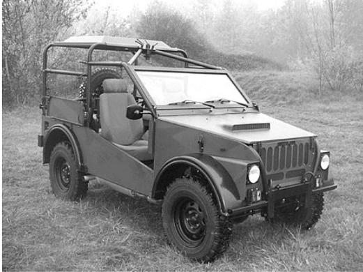
Above: The A3F as operated by the French airborne with cloth top and rollbars. (Photo: Panhard)
