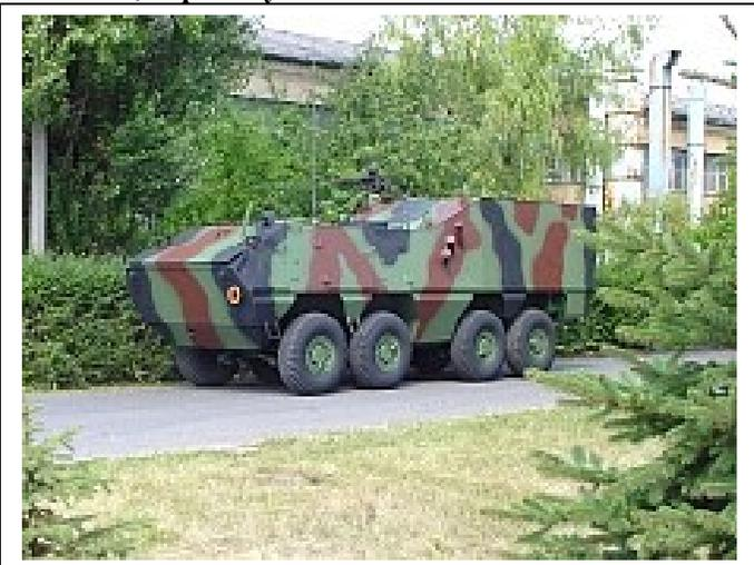
Above: Lynx M98 with raised fighting compartment for firing a mortar from the vehicle. (Photo: WZM-5)
