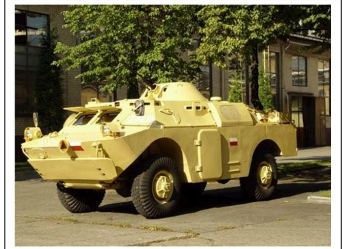
Above WZM-5 Jackal with extra air-conditioning for use in the mid-east. (Photo: WZM-5)
