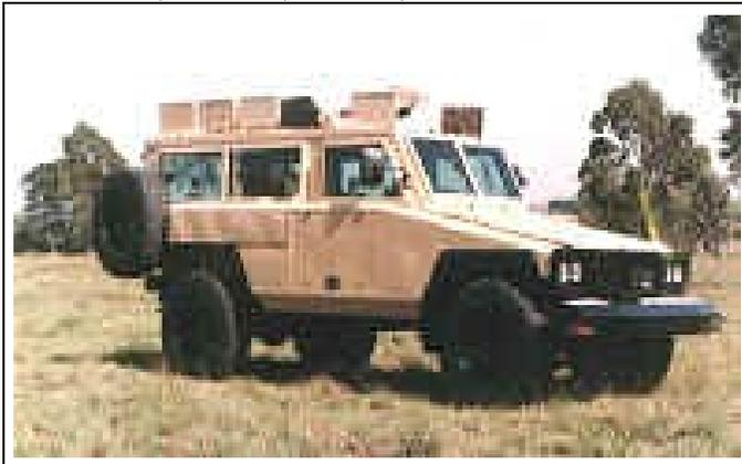
Above: 4x2 Mamba I based on stock Toyota truck components. (Photo: Mechem Ltd)
