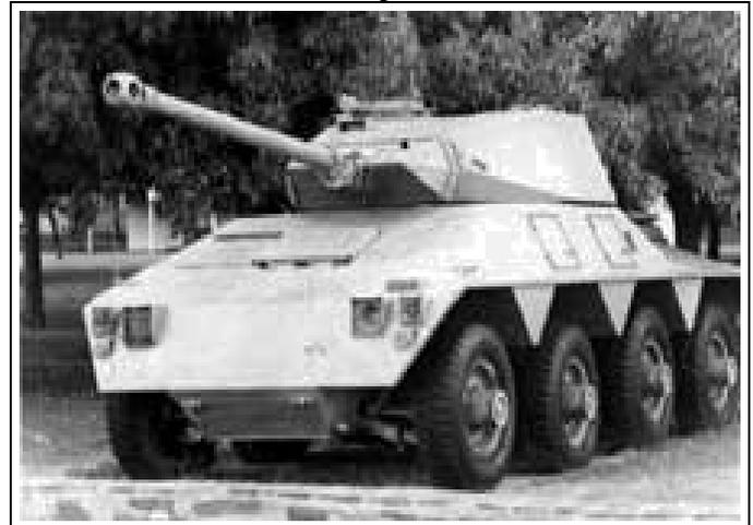
**Remarks:** This test-bed was built around a Saracen Armored Personnel Carrier (APC) side wishbone and torsion bar suspension and bevel box drive line system. The test-bed was built by Sandock Austral (Pty) Ltd in Boksburg circa 1979. The test-bed was to validate vehicle design features such as; suspension, soil mechanics, and large caliber gun firing stress mechanics. Firing trials were carried out with the muzzle brake fitted and removed from the 77mm cannon.
