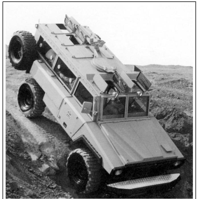
Drive, 4x4. Armor, protected up to 7.62mm or 14 kgs of TNT. NBC Protection, No. *Armament:* (1) .50 cal HMG. Elevation, manual. Traverse, manual. *Capacity:* Fuel, diesel.
