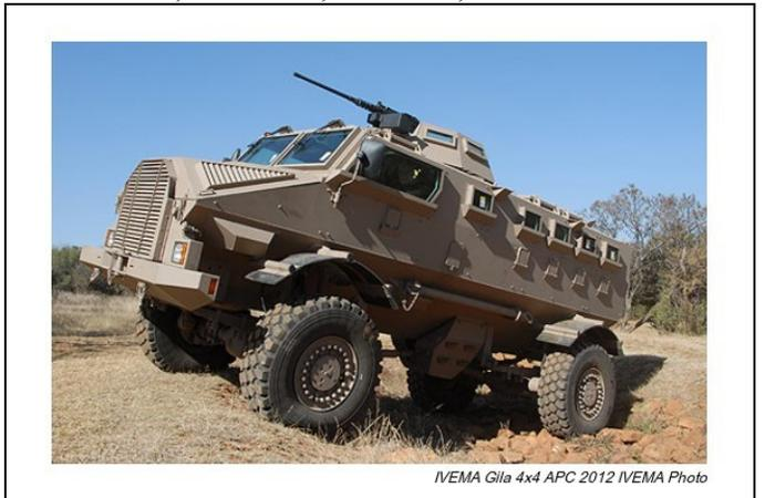
Above: In an effort to meet the demand for new vehicles similar to the Casspir, IVEMA has produced a near clone to the original vehicle. The vehicle does feature a new engine and running gear, along with a redesigned interior. An Anti-Aircraft/Anti-Tank mounting as well as a Police/Interior Security design has also been developed. (Photo IVEMA)
