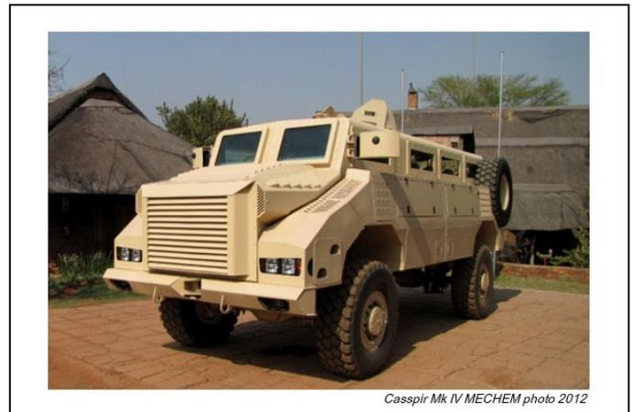
Above: Along with the Casspir Mk II (New Build), MECHEM has also developed a follow-on vehicle incorporating new technology and design for mine-resistant vehicles. (Photo: MECHEM).
