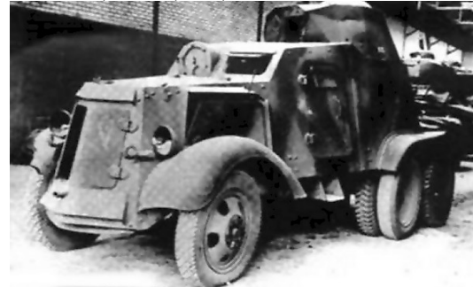
Above: Automilladora Chevrolet. This was a Spanish copy of the Russian BA-3 but on a Chevrolet chassis.
