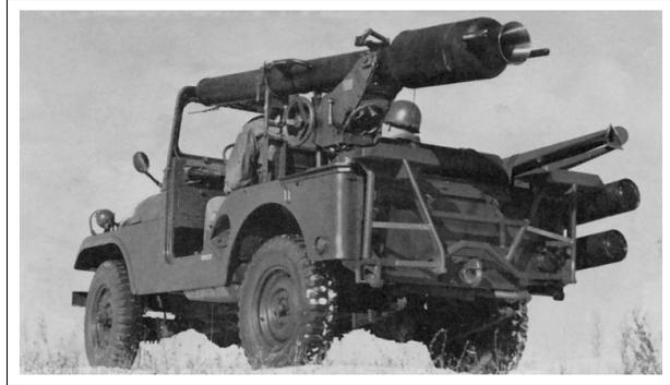
Above: M38A1D with BGAWS M29. Note weapon group was usually mounted on the vehicle right hand side. (Photo: US Army)
