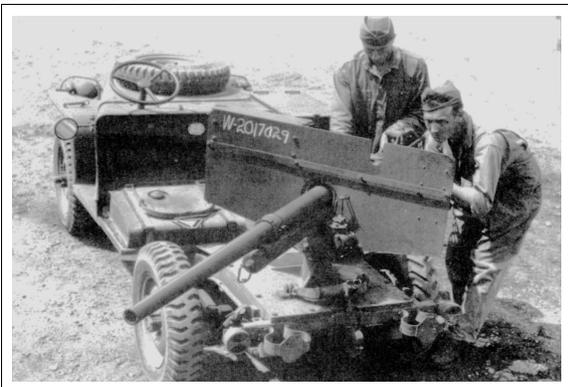
Above: Modified Bantam BRC 40 firing to the rear. As well as the mount for the 37mm gun, the revised position for the steering wheel can also be seen.
