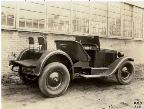
**Remarks:** Armored windshield and radiator. Tested at APG from May to September 1932, the vehicle was found satisfactory and a recommendation was put forward that light scout cars be made by modifying commercial phaeton models.
