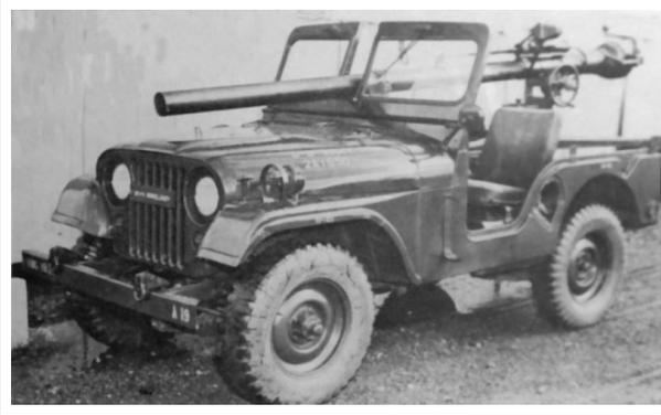
Above: M38A1C with Rifle: 106mm, M40A1 with Mount Rifle: 106mm M79. This combination was to become the standard for the M38A1C. (Photo: US Army)
