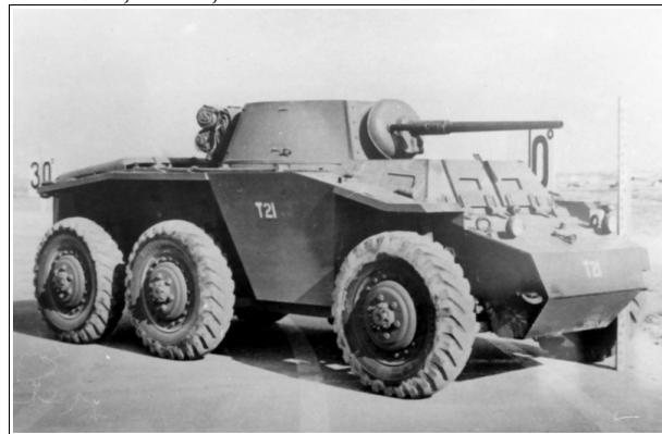
Above: The Studebaker T21 had a non-powered front axle so was actually a 6x4 vehicle. (Photo: US Army)
