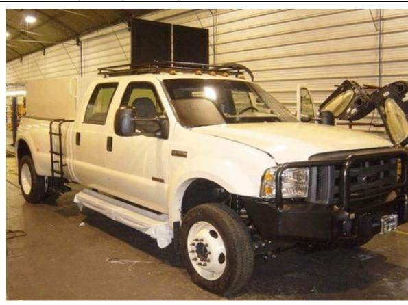
Above: The Lasco Group Gridiron Security Vehicle. Gridirons are protected to NATO Level B-6 (able to withstand up to 7.62mm rounds). (Photos: Lasco International Group)
