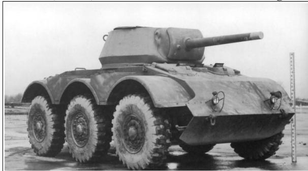
**Remarks:** With the closing of the T19 Armored Car project, the only T19E1 pilot vehicle was modified at the request of Tank Destroyer Command. The 75mm gun M3 was mounted in an open circular turret and fitted to the chassis as the Carriage, Motor, 75-mm Gun, T66. The circular turret was later replaced with a more oval shape allowing extra room for the crew to function. Although the vehicle showed promise, Tank Destroyer Command lost interest and the project was canceled in November of 1942.
