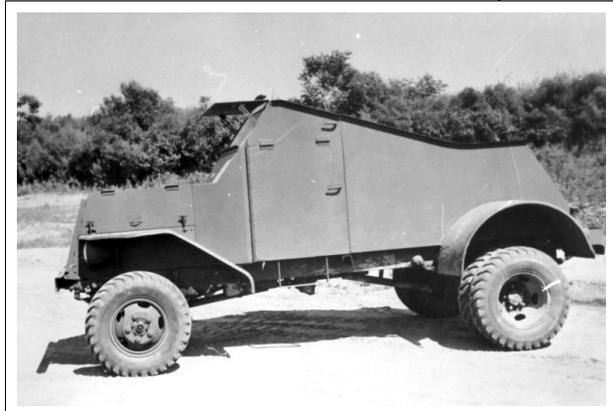
**Remarks:** A private venture by Chrysler to produce an inexpensive and quick armored vehicle on an existing commercial chassis. The armored body was bolted to the top of a Dodge 1/2-ton 4x4 chassis. The vehicle proved to be too narrow and had a very high center of gravity. The same vehicle was later modified with an armored cab and a cargo body at the rear, but no orders were ever placed.
