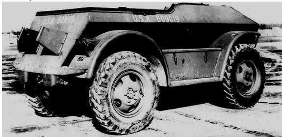
**Remarks:** Based on the 37mm Gun Motor Carriage T8, with the addition of an armored, open topped body, no production undertaken, circa 1941-42.
