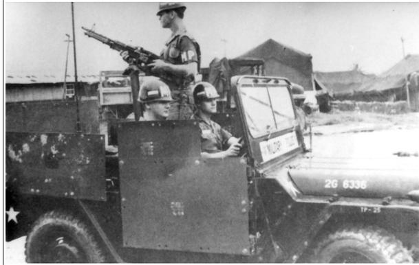
*Above: Typical of the field improvised armor fittings used on the 1/4-ton, this conversion used salvaged armor plate and ingenuity, along with almost no protection from the front. (Photo: US Army)*
