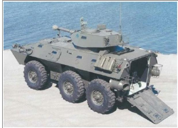
Above: LAV-300 Mk II with 90mm cannon turret with optional water jets. (Photo: Textron Systems Marine & Land Operations)
