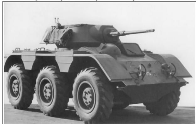
Photos (Above): M38 Wolfhound with original 37mm armed turret. The dome shaped armored hatch over the driver's compartment was hinged and moved as a unit to the driver's right. A canvas hood with plastic windshield could be used with the armored hatch in the open position. (Photos: US Army)
