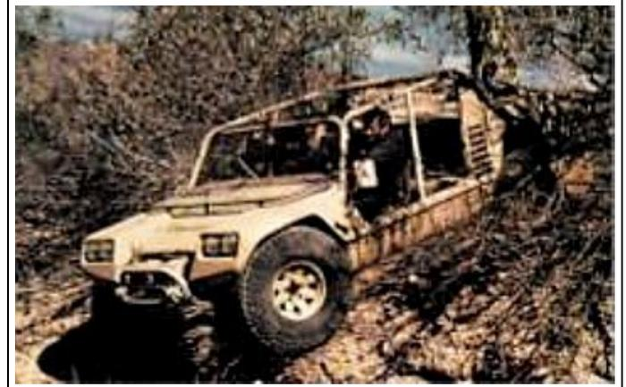
**Remarks:** Designed to fit the US Army's then current requirement for a Combat Support Vehicle (CSV). A rear engine design, development was halted in favor of the front engine HMMWV requirement.
