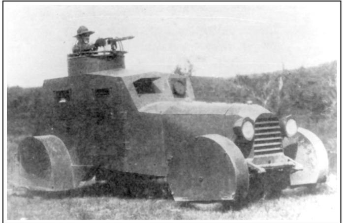
**Remarks:** An independent project, the 112th Cavalry vehicle was designed and built by Cpt. John B. Dunlap. Armament: (1) .30 cal. machine gun. Elevation, manual. Traverse, 360 degrees. Crew, 3-4. Engine: Type, gasoline. Location, forward. Cooling, liquid. Transmission: Type, manual. Suspension System: Type, leaf spring. Steering, front axle. No of wheels, 4. Performance: Speed/Land, 70 mph (112 km/h). Drive, 4x2. Usage: US Army, trial vehicle only.
