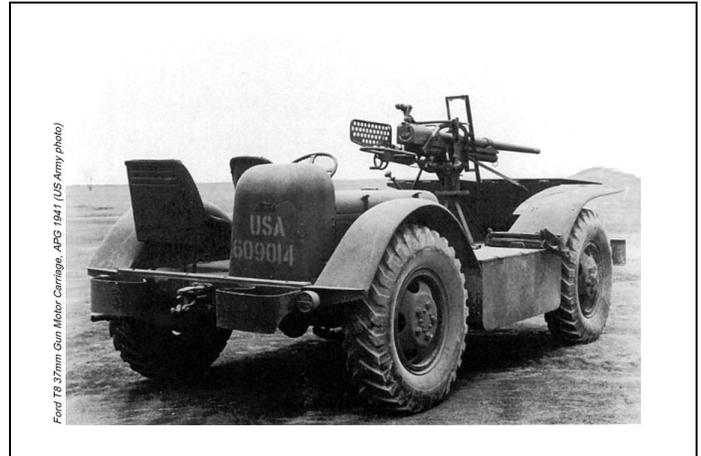
**Remarks:** Ford, "Swamp Buggy", 37mm gun fired forward, 4x4, circa 1941. Fifteen vehicles were built and tested. Project ended in favor of the 37mm Gun Motor Carriage, M6. Two vehicles were later modified into the Observation Post Tender T1 & T2 and at least a few vehicles were bought by the Dutch for the Neatherlands East Indies.
