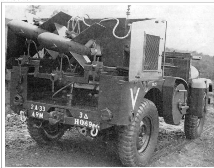
*Above: M38A1 fitted with three French SS10 Anti-tank Missiles.*
