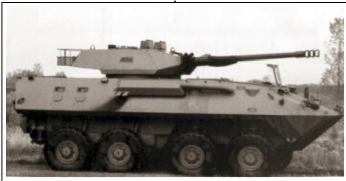
*Above: USMC test vehicle fitted with a 90mm armed MECAR turret.*
