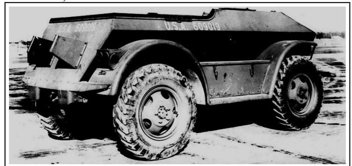
**Remarks:** Based on the 37mm Gun Motor Carriage T8, with the addition of an armored, open topped body, no production undertaken, circa 1941-42.
