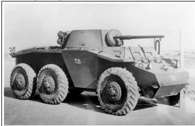
*Above: The Studebaker T21 had a non-powered front axle so was actually a 6x4 vehicle.* **Remarks:** Developed concurrently with the Ford T22 (which became the M8), the Studebaker T21 was a rear-engine design driving the rear two axles, making the car a 6x4. Had it been started earlier, the Studebaker design might have become standard, the Armored Vehicle Board judging the car satisfactory as a reconnaissance vehicle, but engineering problems delayed development and the T22 (M8) won out.
