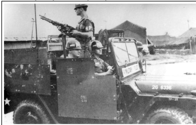
Above: Typical of the field improvised armor fittings used on the 1/4-tons, this conversion used salvaged armor plate and ingenuity, along with almost no protection from the front.
