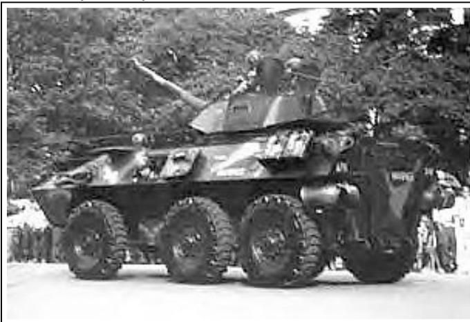
*Above: Philippine Marine LAV-300 90mm Fire Support Vehicle. Remarks: An upgrade from the original Commando V300 developed in 1978, the LAV-300 was chosen by the Philippine Marines when they couldn't get the tracked LVTP7A1. The LAV-300 was chosen because of its amphibious capability and the factory willingness to modify the design to meet their unique needs. Among the changes were the installations of two external waterjets for*
