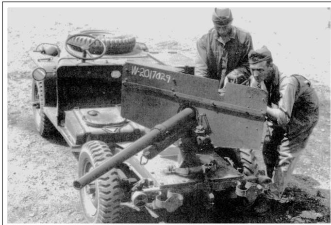
*Above: Modified Bantam BRC 40 firing to the rear. As well as the mount for the 37mm gun, the revised position for the steering wheel can also be seen. Below: the same vehicle with a shortened gun shield and partial covers for the the rear wheels.*
