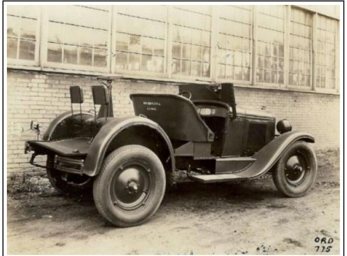
**Remarks:** Armored windshield and radiator. Tested at APG from May to September 1932, the vehicle was found satisfactory and a recommendation was put forward that light scout cars be made by modifying commercial phaeton models.
