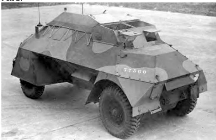
**Remarks:** The second version of the Australian Light Armored Car, Rover. The Mark 2 was shortened by some 24 inches (610 mm) but this didn't actually change the internal volume of the fighting compartment. An open topped vehicle; the Rover had a surprising amount of internal room for the crew and their gear.
