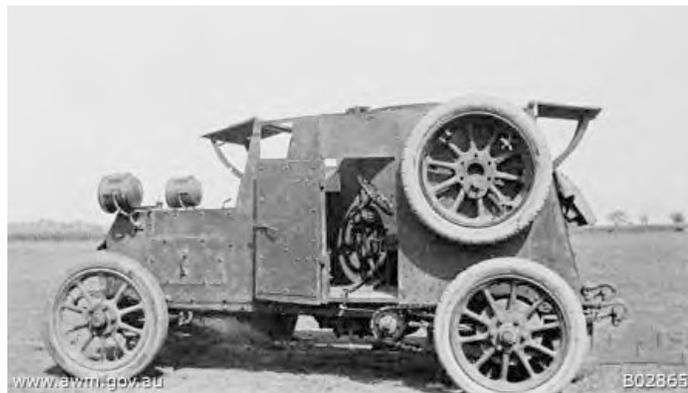
built armored cars produced in Australia on donated car chassis circa 1915. The bare chassis was supplied to the Vulcan Iron Works which applied the armored body. The Mercedes had a full rotating turret and was at armed with a .30 caliber Colt machine gun. *Usage:* Australian Army in the Middle East. *Manufacturer:* Mercedes/Vulcan Iron Works.
