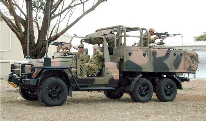
**Remarks:** Australian Army Mercedes-Benz G-Wagon 6x6 Surveillance Reconnaissance Vehicles (SRV) fitted with a locally fabricated custom weapons suite. Under Phase 3A of the projected vehicles on order, approximately 200 SRVs will receive front and rear weapon mounts.
